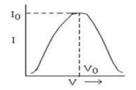
The variation of current with frequency of a.c. source in series LCR circuit
